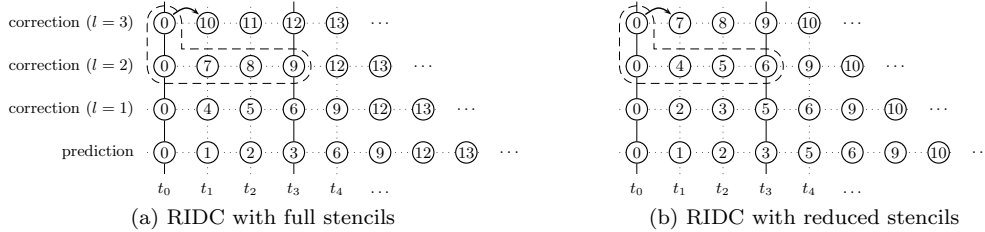
Fig. 3.2: Starting the RIDC4 algorithm. Each number indicates the step in which the corresponding value of f(\eta) is computed. Here M = 3 and in (a) the third correction waits M^2 = 9 steps. In (b) the third correction waits for \frac{M(M+1)}{2} = 6 steps.
